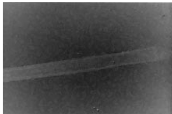
Figure 22. TEM image of a MoS 2 nanotube with arrested growth of a few sulfide layers inside the core of the nanotube that is observed on both sides of the nanotube.
