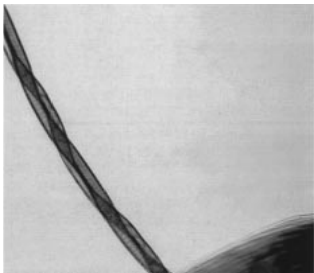
Figure 12. Two entangled spiral WS_2 nanotubes (bundle of 2 coils). 38
